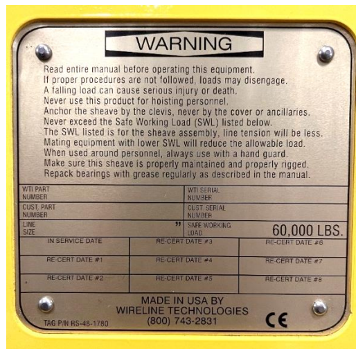
Inspection Tag Figure 9
