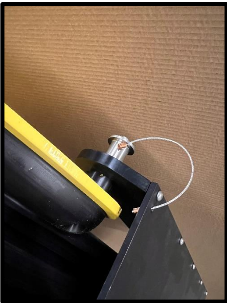
Properly Installed Pin Figure 16
