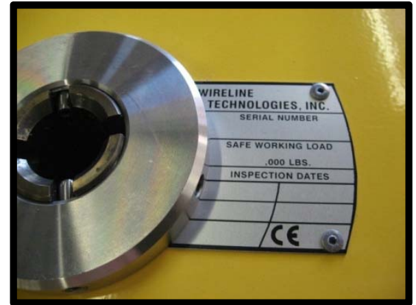
Inspection Tag Figure 13
